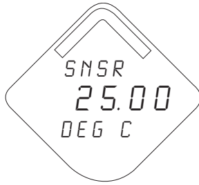
SV Screen - sensor temperature value
