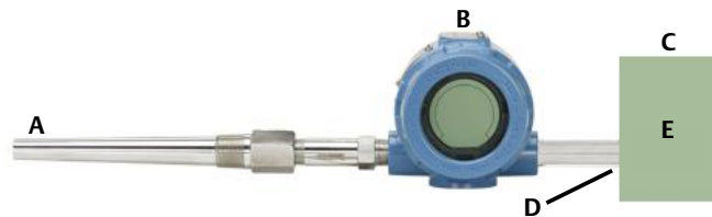
A. Sensor Wires B. Transmitter C. 4-20 mA loop D. Shield ground point E. DCS
